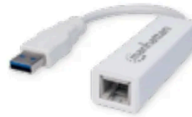
USB 3.0 to Gigabit Network Adapter [506847]* 10/100/1000 Mbps Gigabit Ethernet, SuperSpeed USB 3.0
